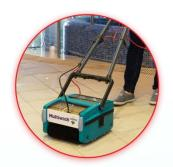
Ideal for cleaning tiled floors and grout as rotary brushes scrub the grout lines clean
